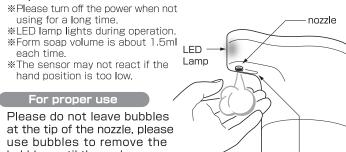
use bubbles to remove the bubbles until the end. If bubbles are left in the nozzle, clogging may result.
