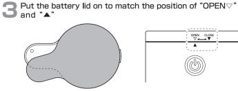
As per the below illustration, turn the battery lid till "CLOSE ▼" moves to "▲'
